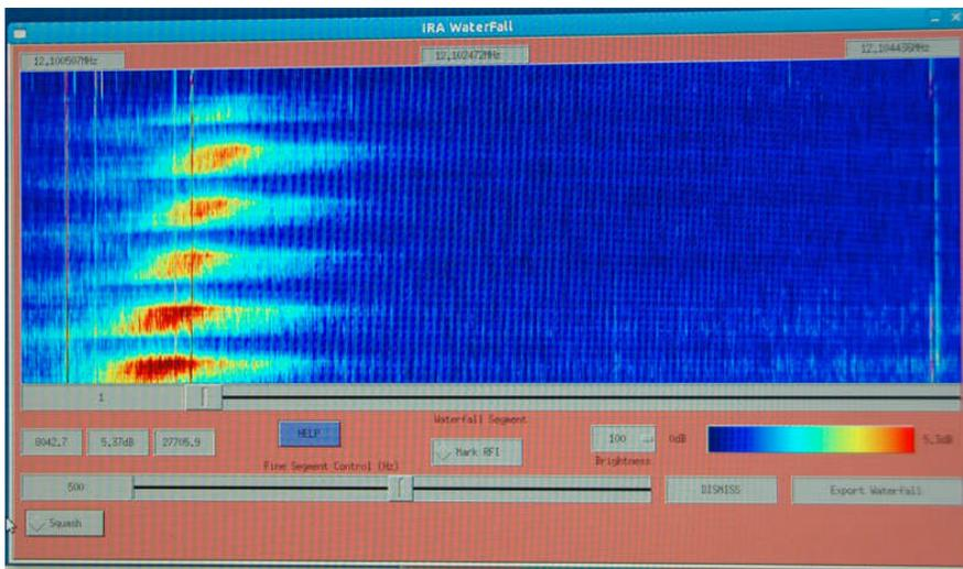
this is the "waterfall", displaying radio emissions as a function of both frequency (horizontal axis) and time (vertical axis). It slowly cascades down the window. (I actually made this image yesterday)
