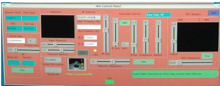
a number of parameters and displays round out the software, which has enough sophistication to handle two receivers in interferometer mode.
