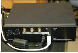
Finally, we get to the receiver, a not-very-impressive box about 8" x 7" x 2", with no knobs, no lights, and not much inside except a fan and a couple of small electronic circuit boards. (<http://www.ettus.com/products>)
