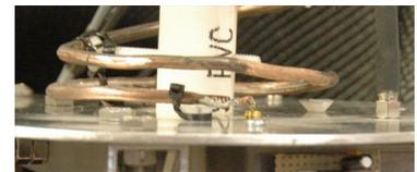
The helix by itself is bi-directional, it literally does not know which end is "up". To tell it, you must put a flat "ground" at one end - the other end is then "up". You could do it as easily as sticking one end in the (moist) ground, but then you could observe only straight up - rather limited. The solution is to place a metal plate (the "ground plane") at one end, and make sure that it is connected to whatever passes for an electrical ground in the system.
