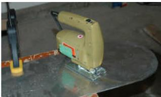
Making the ground plane was fairly straightforward, once I confirmed that my ancient jig saw with a metal-cutting blade would do nicely on the 1/8" aluminum sheet I found at Knox Mountain Metals. I already had a hole saw for the centre hole, and aluminum is a lot easier to work than (for example) steel.
