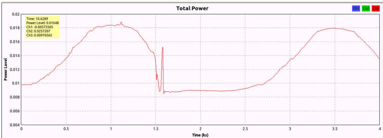
Notice that the shape of the two peaks is the same, and the height is the same above the flat base line. The spikes at 1.6ks (kiloseconds) result from my shifting the dish to point just ahead of the Sun. The flat line centred on 1.7ks shows the base for the peak at 3.5ks, and also the very slight rise of the side lobe at 2ks.
