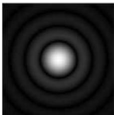
This is seen in well-built optical telescopes, the Airy Disk. The same effect causes side lobes for radio telescopes, or in the case of a dish, concentric rings of reduced intensity.
