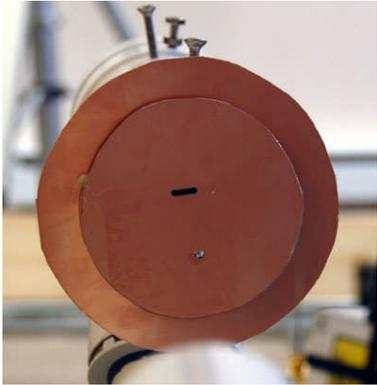
No feed is perfect, they are all a compromise between the two competing requirements, and so a feed has a quality, an "illumination efficiency", that shows the overall effectiveness at receiving the signals the dish collects. A typical feed has an efficiency of about 50-70%; my first effort, called a "patch feed" (left), is probably less than 50%, so the signals I have been getting from the Sun are not as good as if I used a different feed.
