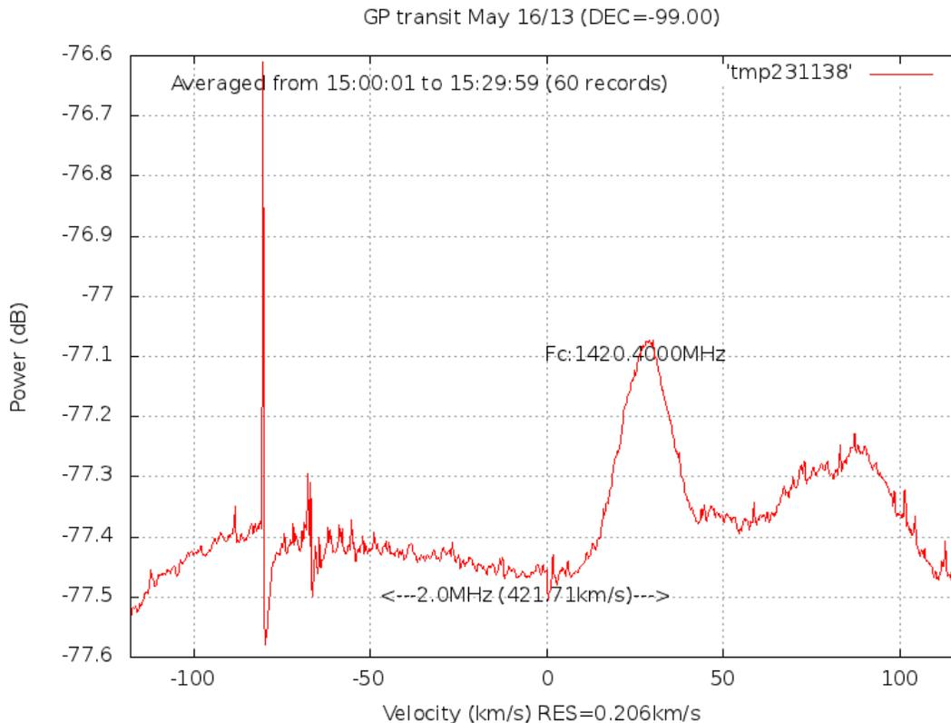
This plot shows the power level on the left, with the main peak at about 30km/s about 0.4dB above the noise floor.
